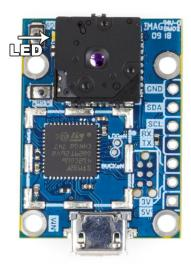
**LED:** When plugged in to micro-usb power and a Lepton is inserted in the socket LED will flash slowly. When video is being transmitted to the viewing program, LED will flash more rapidly.
