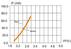
FIG.1 FORWARD CURRENT VS. FORWARD VOLTAGE.
