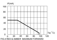
DC CURRENT VS AMBIENT TEMPERATURE (Tjmax=105°C)
