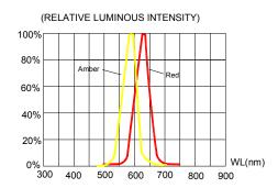
FIG.5 RELATIVE LUMINOUS INTENSITY VS. WAVELENGTH.
