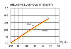
FIG.2 RELATIVE LUMINOUS INTENSITY VS. FORWARD CURRENT
