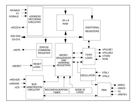
Figure 1 - COM20022I Internal Block Diagram
