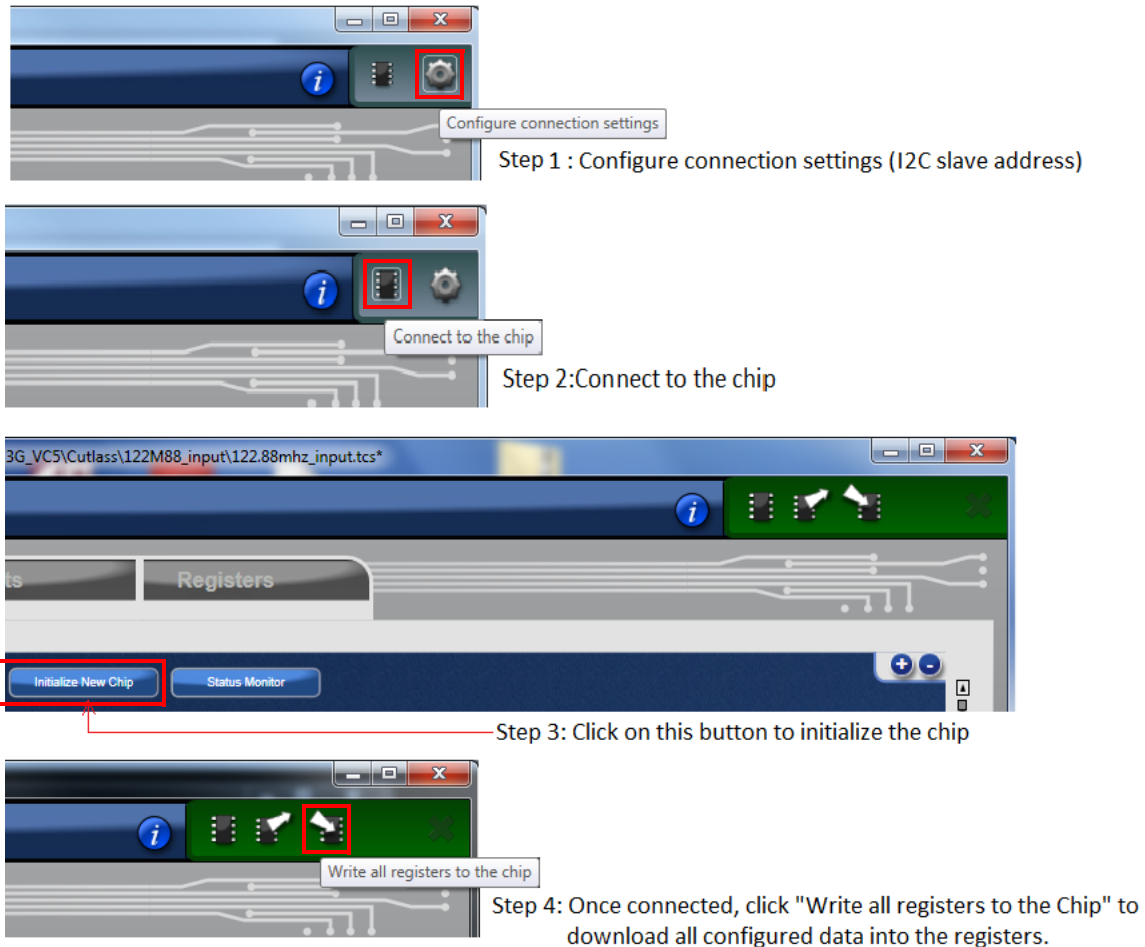
Figure 18. Steps to Making Connections and Writing to the Board
