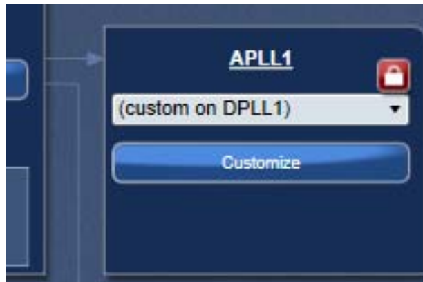
Figure 12. APLL1 Parameters for VCO = 614.4MHz
