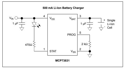
FIGURE 1-1: Typical MCP73831 Application.
