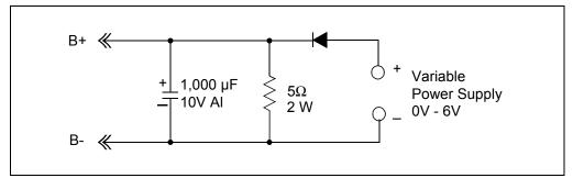
FIGURE 2-2: Simulated Battery Load.
